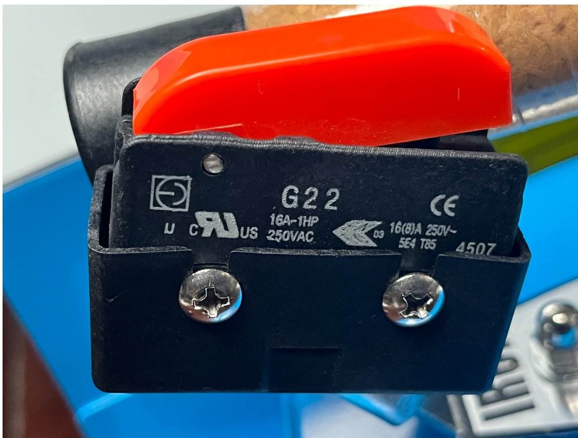
Iron steam-control microswitch in The Workshop Ledger ST-750 reference unit. Pressing the red hand control mechanically actuates the microswitch; the installed switch carries a visible G22 marking.
