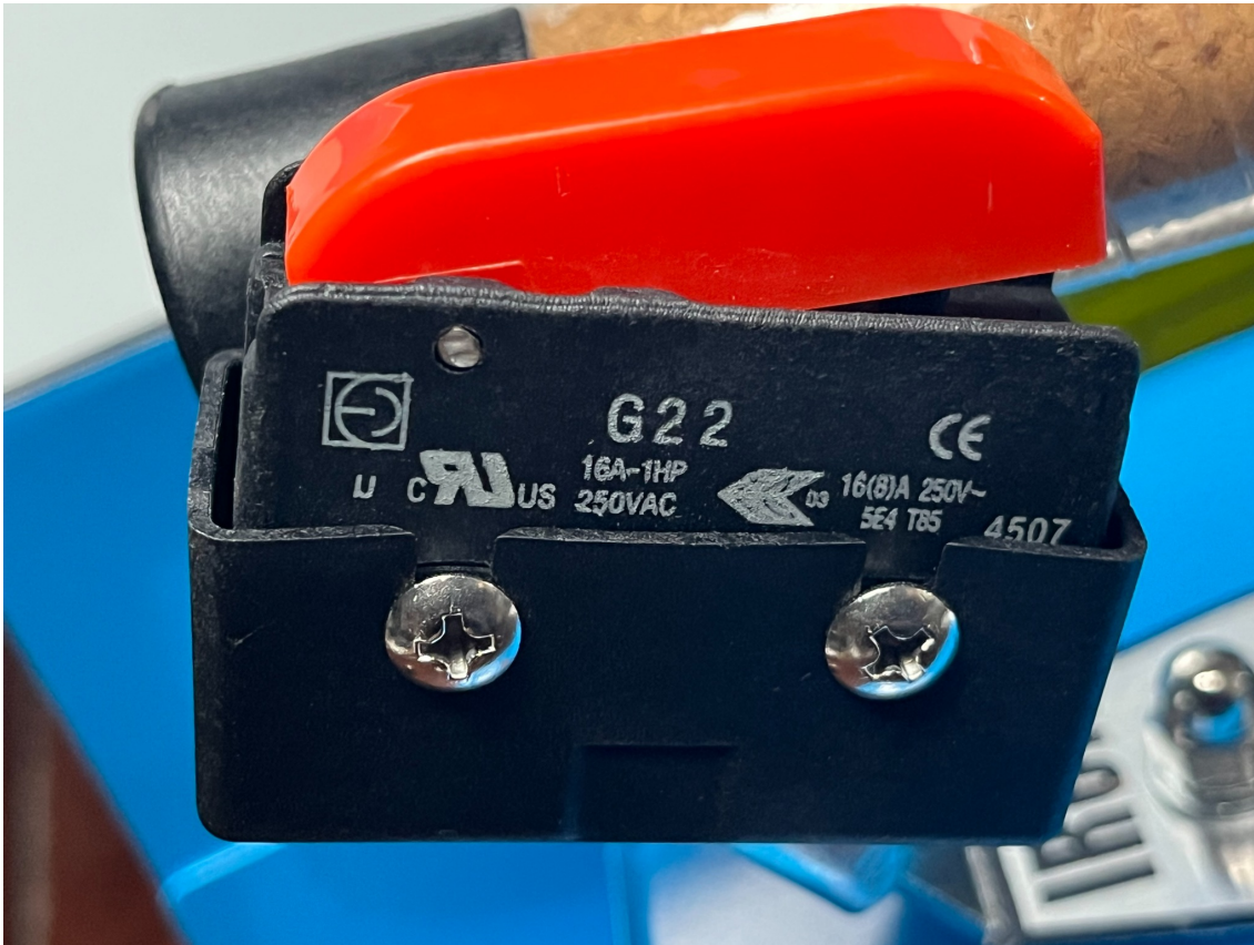
Hand-operated steam control on the ST-750 heated iron. The red control actuates the internal microswitch; the installed switch is visibly marked G22.
