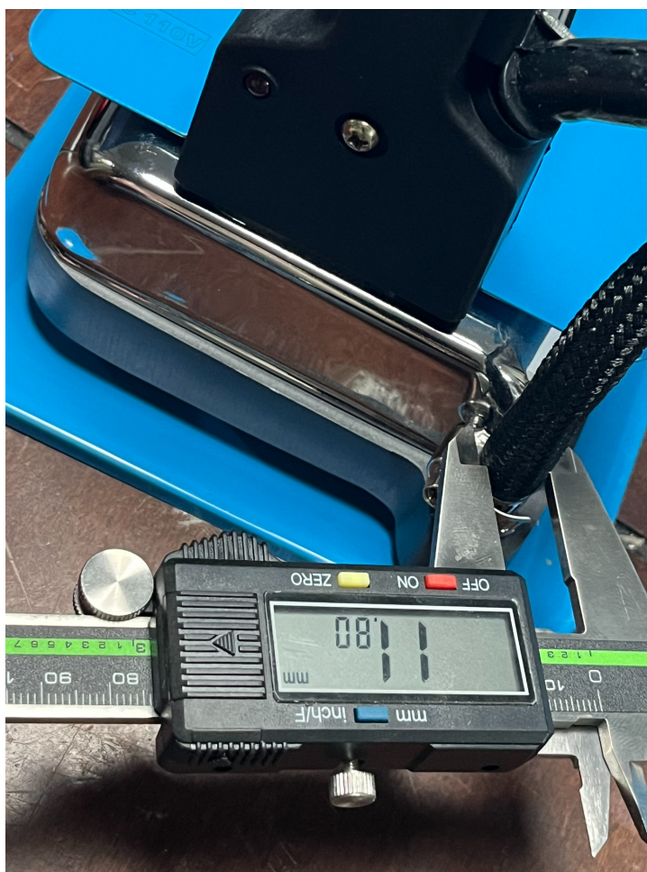
Direct measurement of the installed flexible steam hose on The Workshop Ledger ST-750 reference unit. The digital caliper indicates an outside diameter of 11.80 mm.
