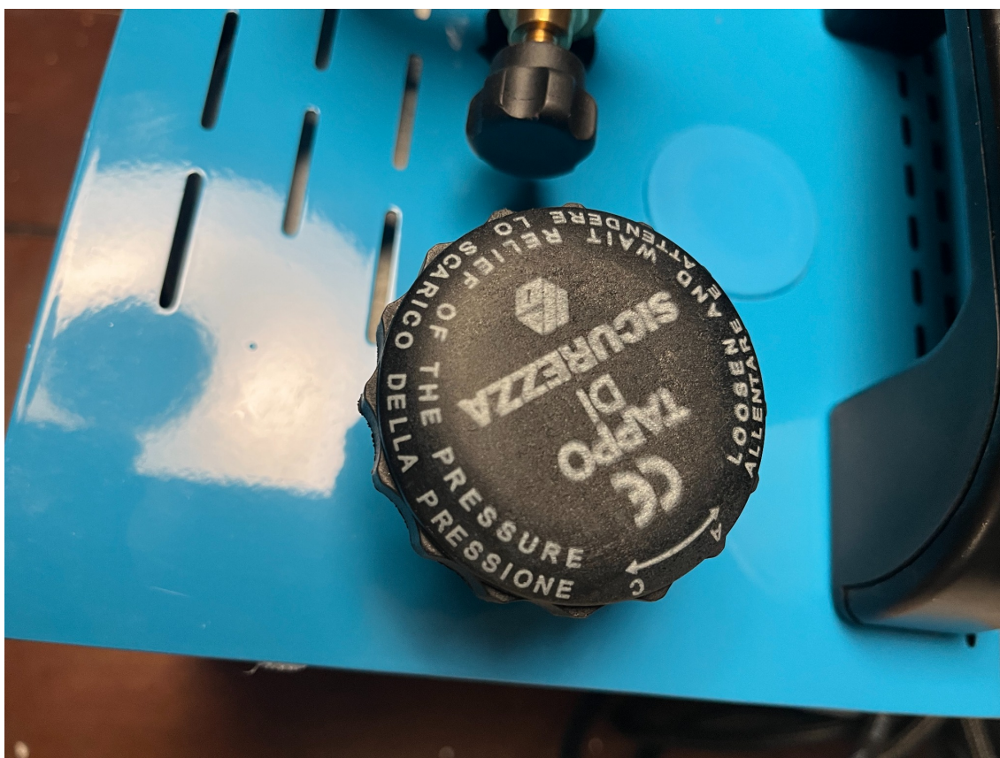
Boiler fill cap on The Workshop Ledger ST-750 reference unit. The cap is marked with a warning not to open it while the boiler is under pressure.
