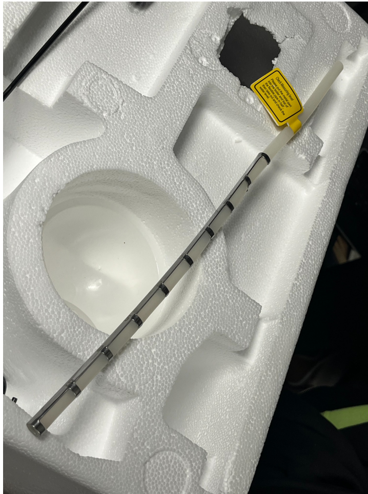
Water-level dipstick supplied with The Workshop Ledger ST-750 reference unit. The metal measuring portion incorporates multiple stepped or marked level positions.
